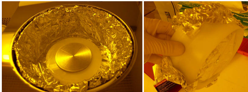
Figure 3: Aluminum foil is used to keep the spinner head area clean.
